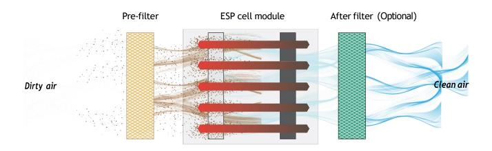
When contaminated air passes through the IVOLTAIR<sup>™</sup> unique designed advanced electrostatic cell module, containments electric potential and filtration takes place in cell module, Cell needs to be cleaned
